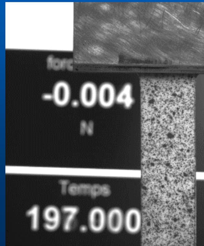
*(Essai de traction simple 3S)*
